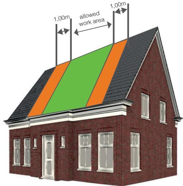
The RSS system is used with a fence 3 metres in length. If installed according to these instructions, it is suitable as temporary edge protection as described in EN 13374 +A1 2019 Class C for roof gradients of up to 60 degrees as long as the fall height is no more than 5 metres. In Class C situations (see drawing) **the hooking bar** is mandatory. Protective fences must extend beyond the work places to be secured at least 1 meter.
